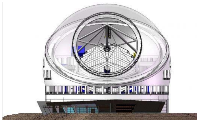
Dome Home: The 66-meter diameter "Calotte" style dome protects the TMT from high winds atop Mauna Kea, while also allowing full range of motion. TMT Observatory Corporation
