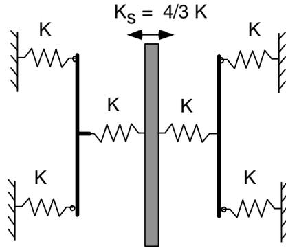
Figure 6. Equivalent lateral stiffness model of the actuator
