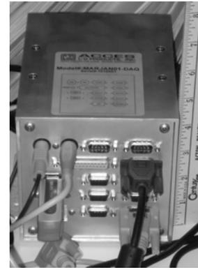
Figure 12. A picture of the PC104 computer that will be used to control the P<sub>1</sub> prototype actuator
