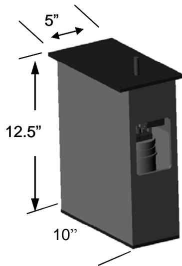
Figure 8. Mechanical envelope of the TMT soft actuator
