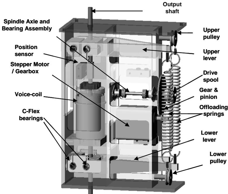
Figure 7. Actual implementation of the TMT soft actuator
