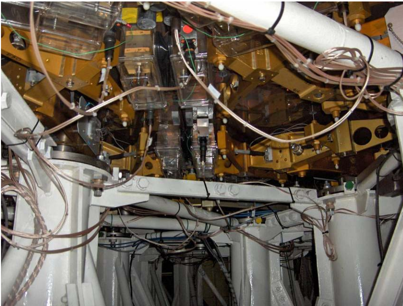
Segment and mirror cell cabling
