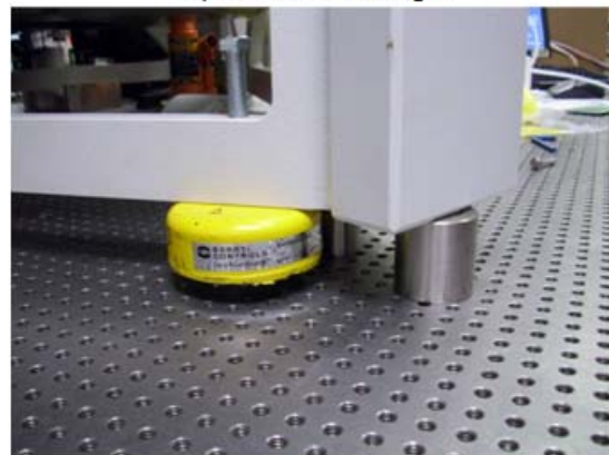
e) Alternative supports for mirror cell triangle, stainless steel post & yellow machinery mount
