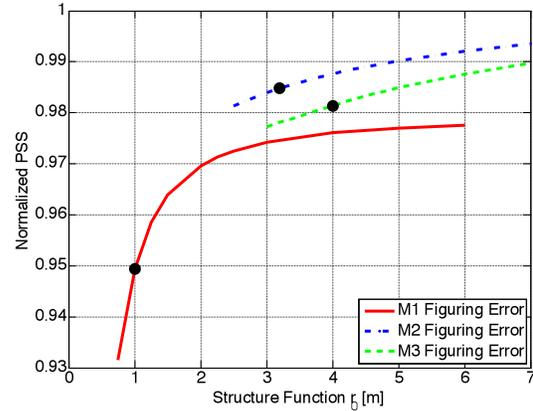
**Figure 8** – Performance sensitivities to mirror shape specifications expressed as atmosphere like structure function characterized by the associated  $r_0$  value. The black dots mark the current mirror specifications.
