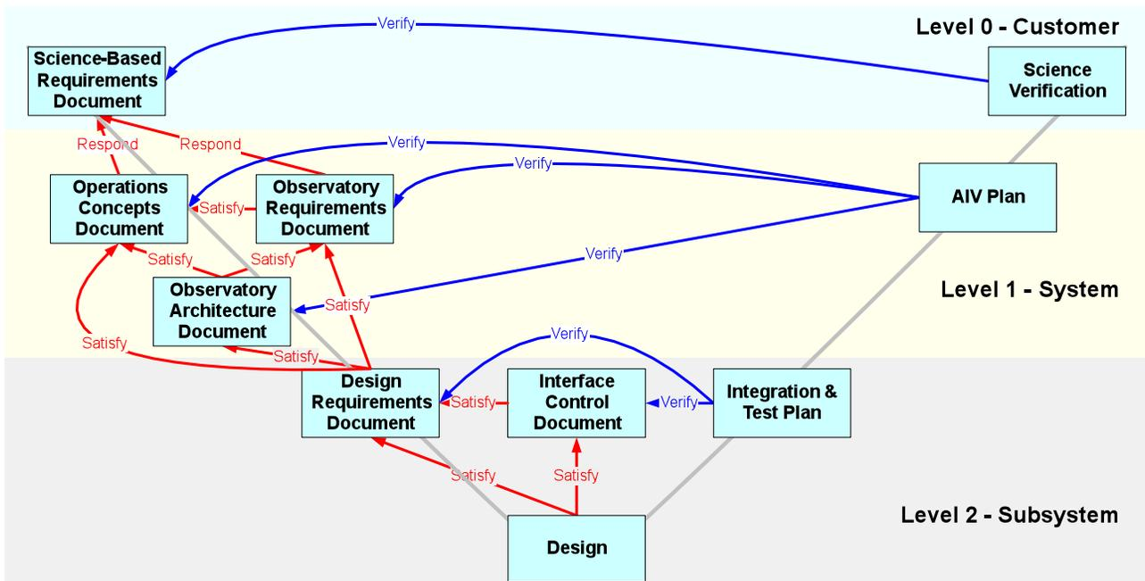
Figure 1 - Systems engineering lifecycle V-diagram for TMT
