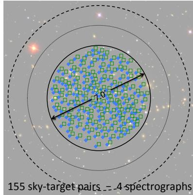
**Top:** Illustrations of the sampling of the TMT focal plane for the Xchange (far left) and fiber fed forms of the WFOS instrument when sky nodding. 7' diameter field is for 4 modular spectrographs with 22" pitch, 100% overlap fiber positioners.
