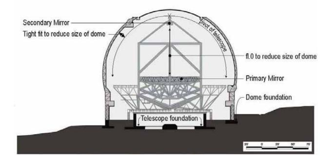
Figure 5-2: Comparison of Observatory Dome Sizes to Telescope Focal Ratios
