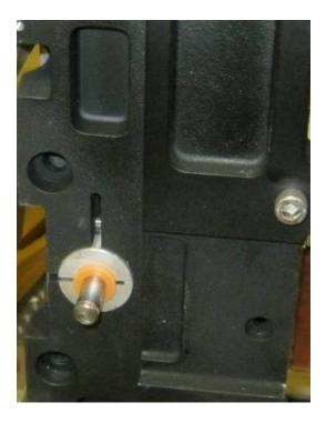
Install the J-20 offload bearings in the spring block, and clamp them in place. The bearings should be inserted until they are flush with the inside radius of the block. (The photo, below, is for actuator #2, but the flexure bearings install in the same location).
