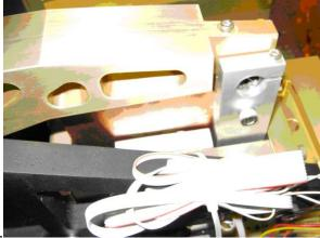
WARNING!!! The magnets to be installed are very powerful. They are attracted to each other and to steel parts with >100# force at short distances. Wear leather gloves when handling and installing the magnets. Use extreme care not to get magnets near steel parts or work surfaces, other magnets, or each other, until they are installed in the enclosure (which closes the magnetic circuit).
