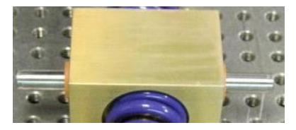
Assemble the spring block, springs, upper and lower connection blocks, pivot blocks and connecting rod as shown on a flat surface. The blocks must all align after torquing the screws tightly.
