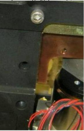
Mount the encoder head to the encoder bracket, and mount the bracket to the housing. To avoid scratching the encoder scale, use a soft cloth to keep the parts from touching until the screws are tightened. (For production, the encoder would also be installed earlier in the process, and protected until this stage by a few layers of wrapping paper and tape.)
