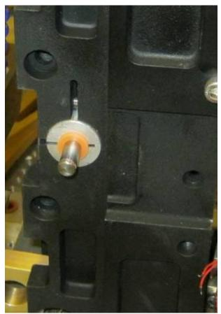
(The pivot pin adapter shown in the picture is not required for the current housing design. You can see one of the two clamp screws extending across the slot above pivot pin; they are accessed from the left hand side of picture. Different spacer washers are used in the current design, installed later). Install the spring block assembly and upper <sup>3</sup>/<sub>4</sub>"flex pivot (TMT-202), but don't tighten the flex pivot clamp screws yet.
