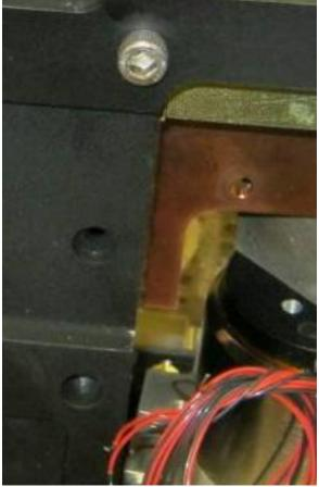
Mount the encoder head (TMT-310) to the encoder bracket (TMT-128), and mount the bracket to the housing. To avoid scratching the encoder scale, use a soft cloth to keep the encoder head from touching the scale until the screws are tightened. (For production, the encoder would also be installed earlier in the process, and protected until this stage by a few layers of wrapping paper and tape.)
