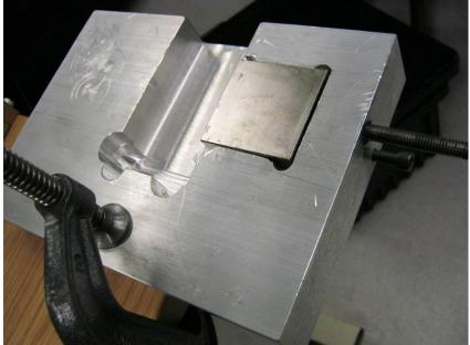
Use the magnet jig to remove a magnet from the stack
