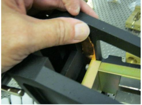
Center the copper plate, attach the second screw holding it in place. Use a  $\frac{1}{2}$ " dowel pin in the upper flex pivot hole, and a  $\frac{1}{4}$ " dowel pin in the lower through-hole, to center the two halves of the vertical linkage. Tighten the two copper plate screws, and remove the pins. Only hand tighten the clevis screws at this stage.
