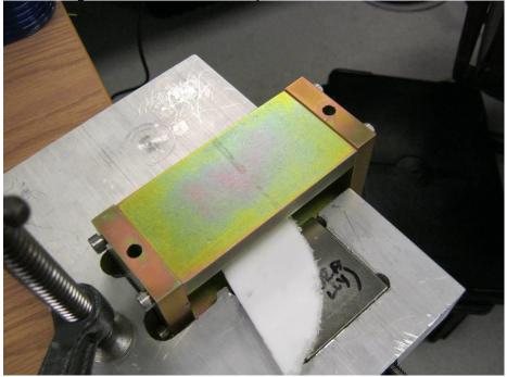
After installation, the attraction of the magnets to the steel plates will keep them in place in the assembly. For production, we would probably use some wicking adhesive, but that's not needed for the prototypes.
