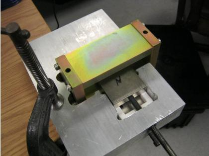
(You can see in the photo the annular square plastic spacer which separates the magnets in the stack.)
