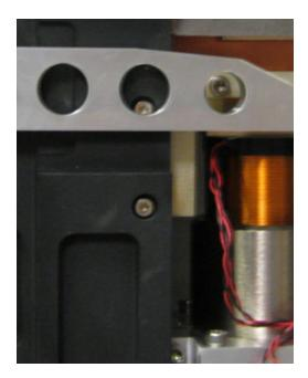
Use the Mercury II encoder alignment tool and verify proper signal over the range of travel of the actuator, and adjust the encoder mounting bracket as required.
