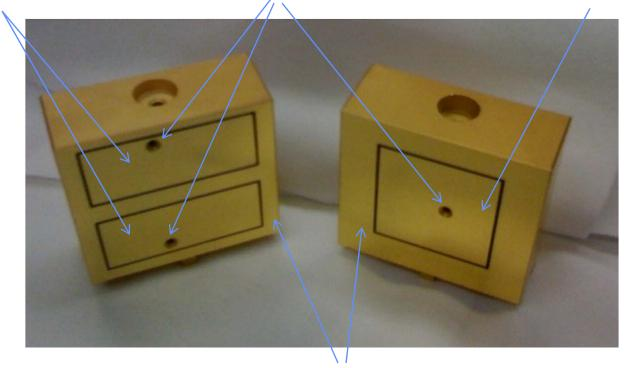
Guard Electrodes (coating on all sides except bottoms of feet)
