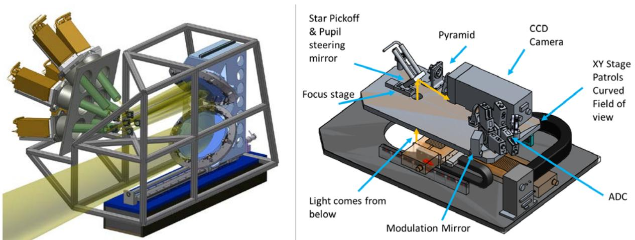
**Figure 7 Wavefront sensor assemblies. Left Trombone & LGS. Right: NGS (NVNW)**
