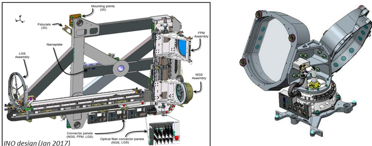
**Figure 6 Left: Source Simulator; Right: Beamsplitter changing mechanism**
