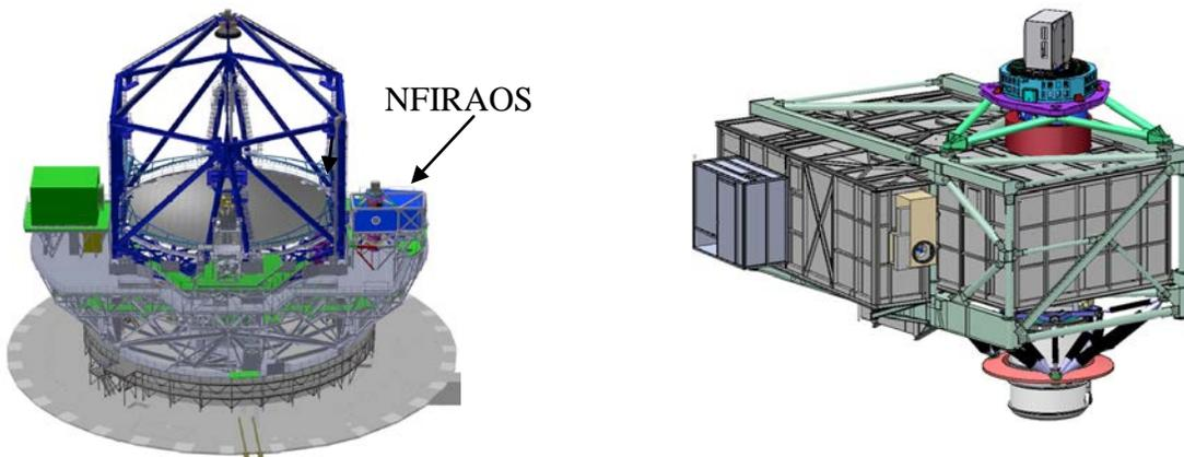
Figure 1 Left: TMT & NFIRAOS; Right: NFIRAOS with client instruments on top and bottom ports
