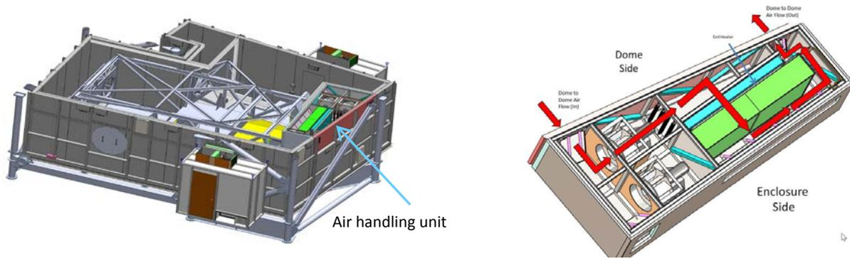
**Figure 4 Left: Thermal Enclosure, and optical table (unpopulated); Right: Air handling unit - defrosting**
