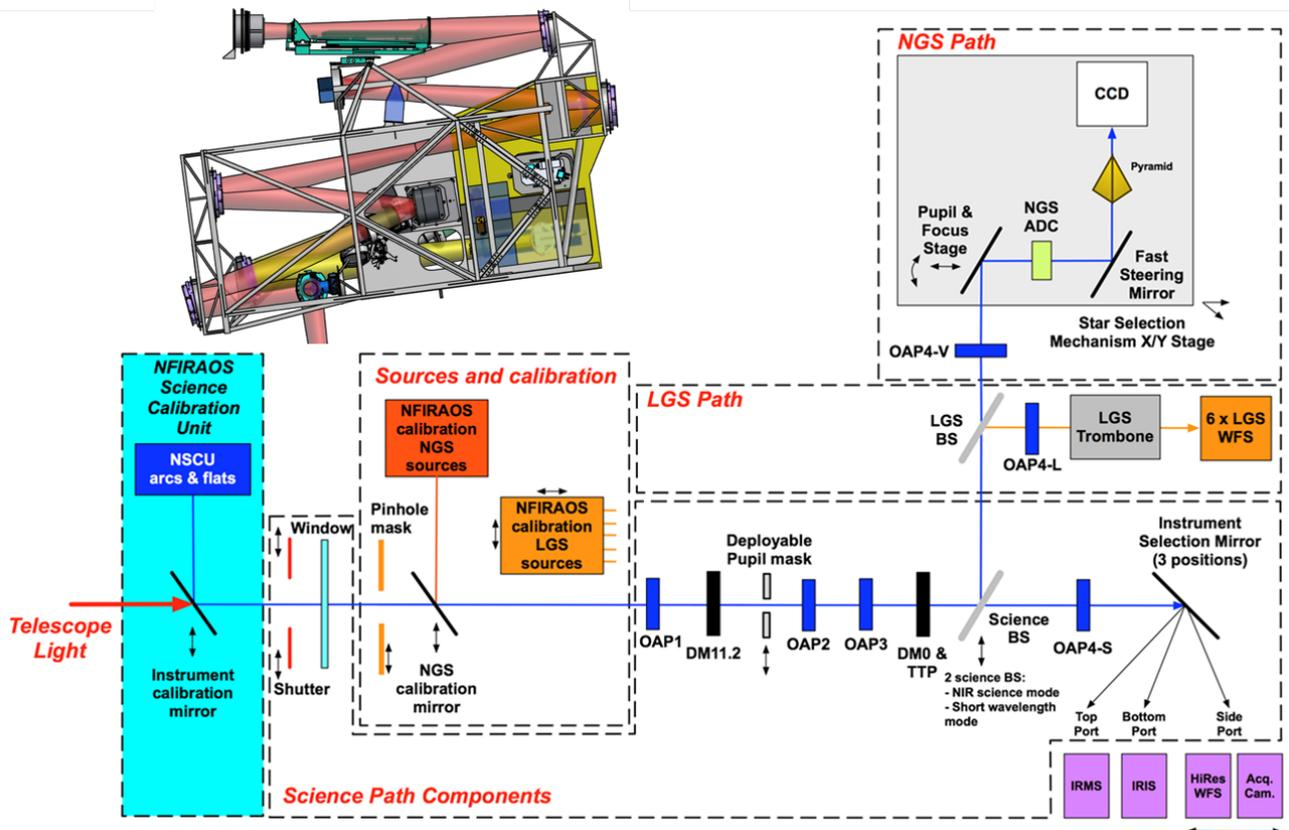
**Figure 2** Block Diagram of NFIRAOS Optics; Inset: Overhead Plan view - Light path is top to bottom.
