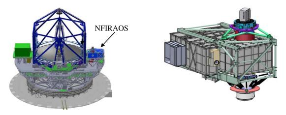
Figure 1 Left: TMT & NFIRAOS; Right: NFIRAOS with client instruments on top and bottom ports
