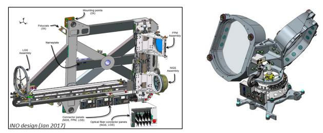
**Figure 6 Left: Source Simulator; Right: Beamsplitter changing mechanism** picture in Figure 6, are a Focal Plane Mask (FPM) with a grid of pinholes, and a Natural Guide Star Assembly with up to
