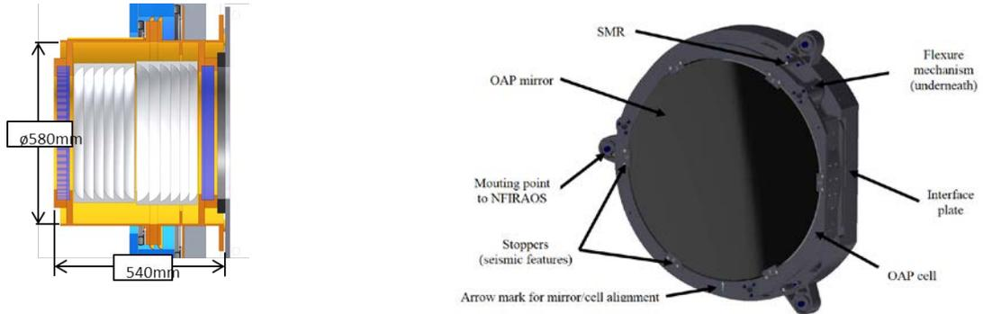
**Figure 5 Left: Evacuated Double Pane Entrance Window; Right Mirror Cell**
