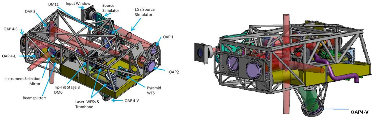
Figure 3 Opto-mechanical table (space frame)
