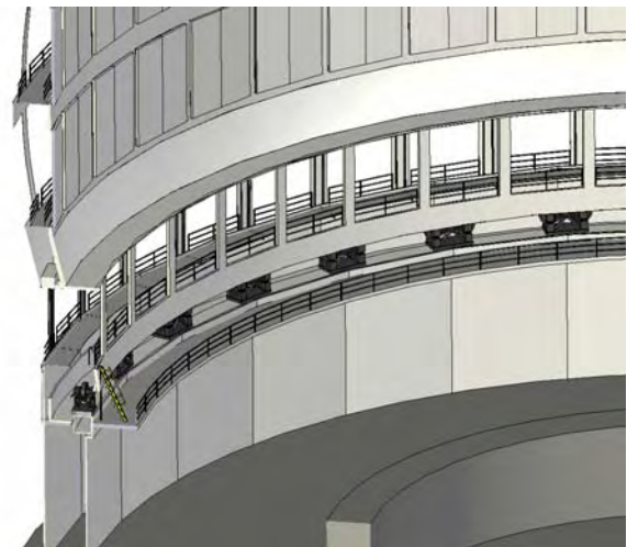
Fig 7-4: Stairs and walkways on the enclosure.
