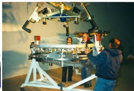
Fig 8-47: The Keck segment lifting mechanism.
