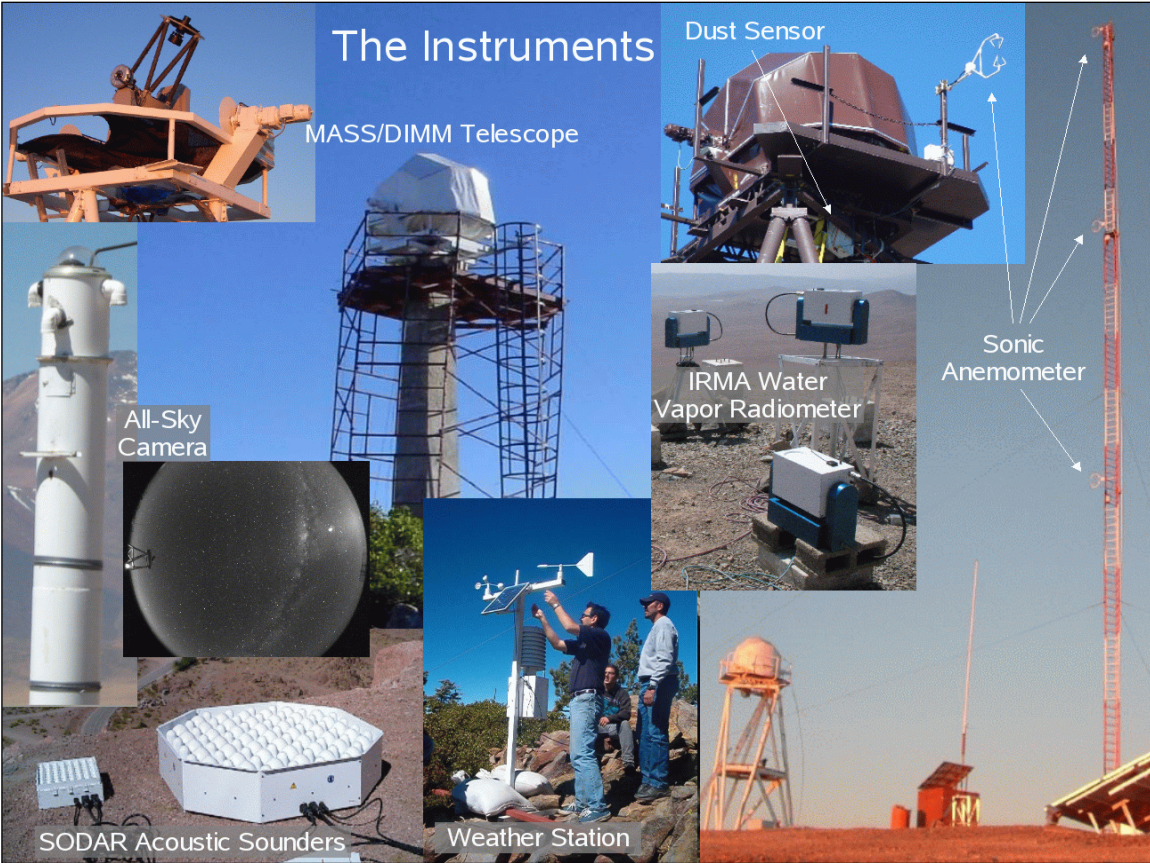
Fig 4-2: The TMT site selection instrument suite.
