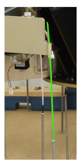
Use green 12" straws (21x) for alignment of SSA with M3 rods
