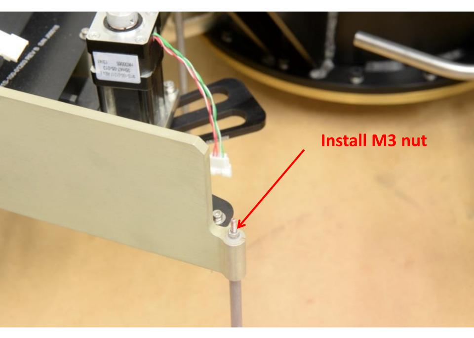
Torque M3 bolts with wrench (~1 Nm – do not overtighten Nylon washer)
