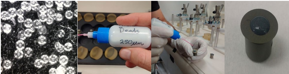
Figure 13. Using Microspheres to Establish the Bond Line Thickness
